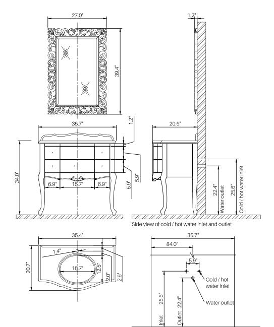
Elevation view of cold / hot water inlet and outlet Plumbing inlets and outlets may vary based on location
