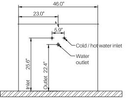
Elevation view of cold / hot water inlet and outlet Plumbing inlets and outlets may vary based on location
